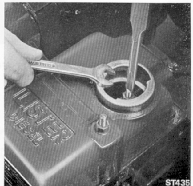
Fig. 39. Adjusting the Decompressor
