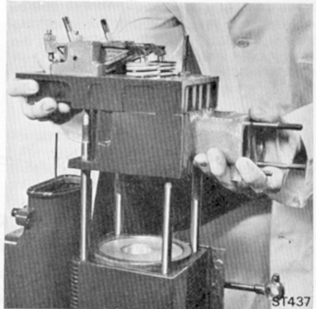
Fig. 41. Removing the Cylinder Head
