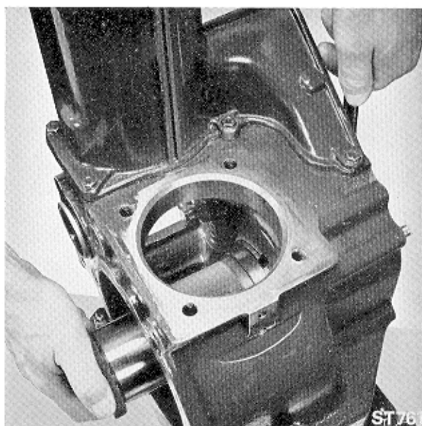
Fig. 131. Fitting Main Bearing
