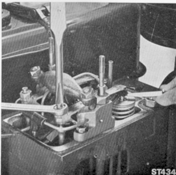
Fig. 38. Adjusting Valve Clearance
