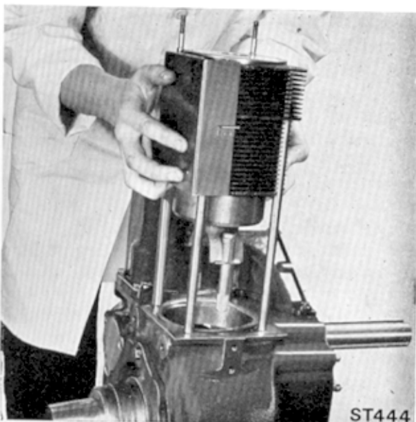
Fig. 48. Removing Cylinder Barrel
