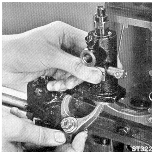
Fig. 22 Removing Fuel Pump
