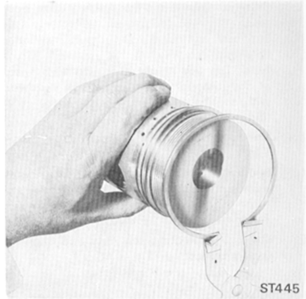
Fig. 49. Fitting Piston Rings
