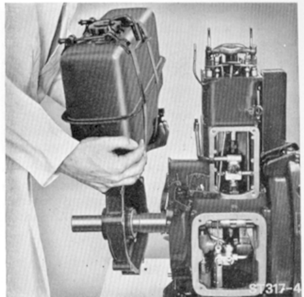
Fig. 50. Removing End Cover and Fuel Tank
