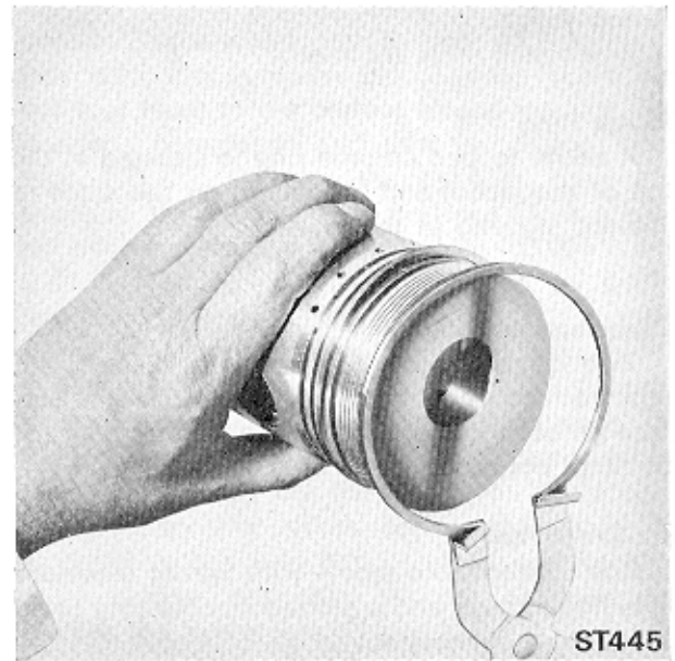
Fig. 79. Fitting Piston Rings
